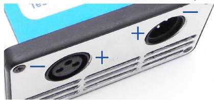
3. Connect the original product charger for the test battery (12V/24V) to the left socket.
