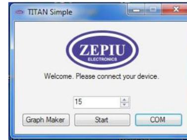
COM - if you do not know the port number com to which the Tester has been assigned, click on this button. The port number will be shown in a new window - enter this number in the Program window and click the middle Start button. After reading Tester data, a new window will appear to save the file. Leave the destination as default, or choose to save somewhere else, but you must give it a filename. The filename must start with "TestA" (e.g. TestA\_battery\_scooter1).
